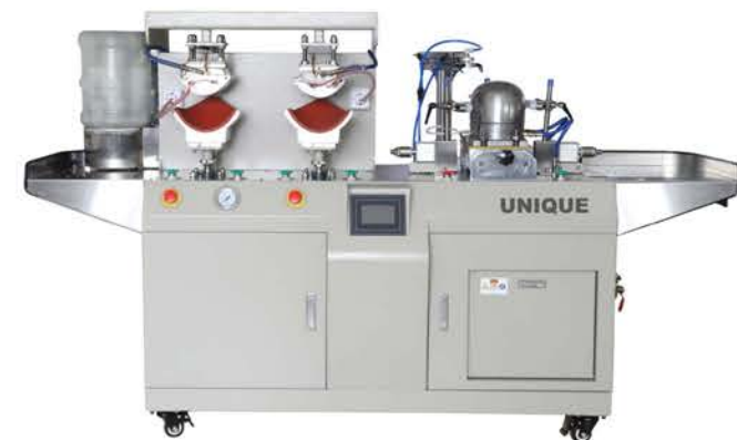
UN-CL1031 Multi-function cap ironing machine UN-CL1031 with cap front panel pressing and ironing UN-CL1032 with cap curved visor blocking and ironing UN-CL1033 with cap front panel pressing, curved visor blocking and ironing
