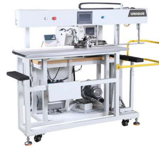
UN1903ASS-L01 Automatic button attaching machine with auto fabric feeding and button feeding 1-20 pcs of buttons can be set. Distance between the first and last button 655mm Suitable for shirt
