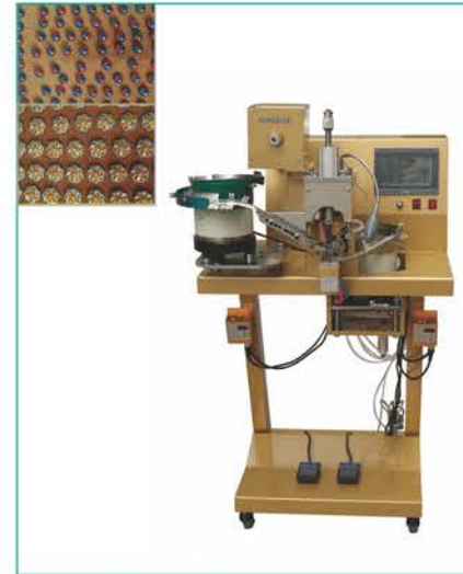
UN-198-E Automatic pineapple nails plastic button attaching machine (both round shape and other shapes for heavy duty)
