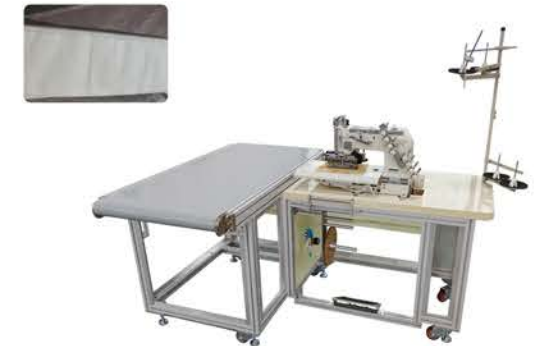
UN-HBJ100 Computer multi-needles curtain sewing machine
