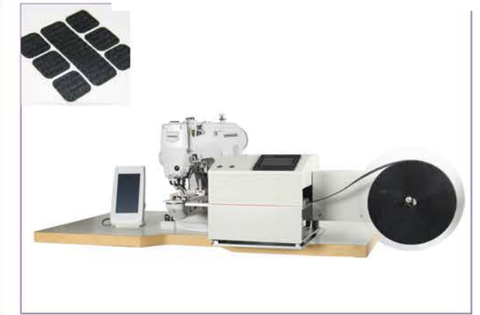
UN436D-AVCB Automatic velcro tape cutting and attaching machine with bottom feed with max. tape size 9*6cm UN342G-AVCB with max. tape size 30*20cm UN326G-AVCB with max. tape size 20*10cm UN430D-AVCB with max. tape size 4*3cm
