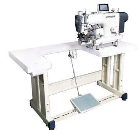
UN63902-WH Automatic jeans bottom hemming machine with lockstitch & chainstitch exchangeable with max hemming width up to 10cm
