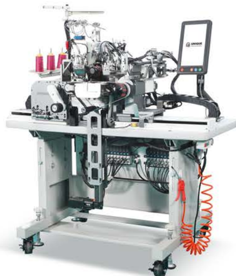
GK-375S Automatic underwear elastic waistband attaching machine
