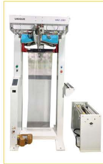
UN-P208E Automatic garment packing machine with auto sealing bag length adjustment UN-P218XE bottom edge can also be sealed
