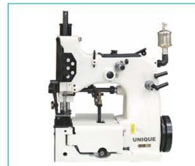
GK35-2S 1 needle 2 thread up and down feed bag sewing machine Stitch length: 9-15mm Max thickness: 18mm
