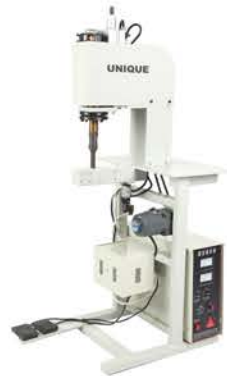
UN-SK Feed off the arm ultrasonic seaming machine (For sleeve seaming without thread stitch) Working Width: 1.5-25mm Production speed: 1-20m/min
