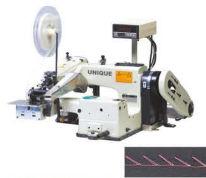
UN370DD-T Direct drive belt loop blind stitch sewing machine - with knife, width adjustable UN370DD Direct drive
