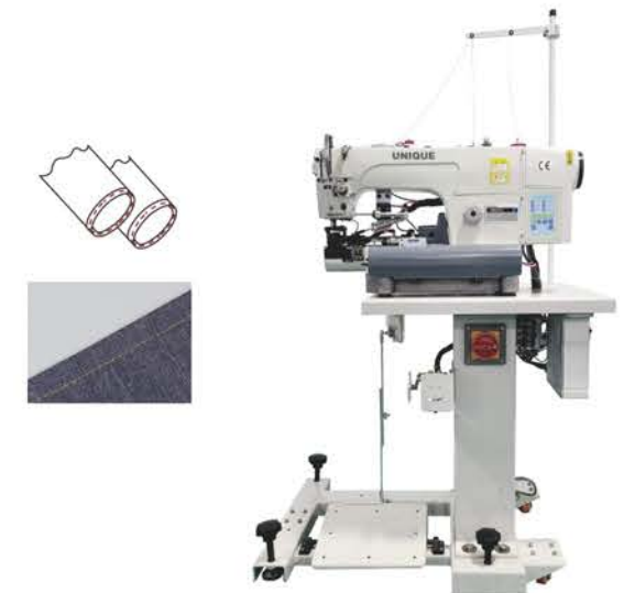
UN63972 Automatic jeans bottom hemming machine with lockstitch & chainstitch exchangeable UN63970 Lockstitch type only UN63971 Chainstitch type only
