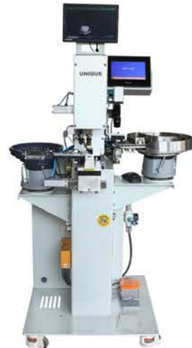
UN9828 Automatic snap button machine It can recognize a series of button image recognition such as letters, special-shaped patterns, striped plaid LOGO, etc.
