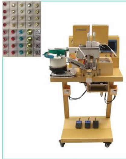
UN-198-9X Automatic plastic button attaching machine (different shapes)
