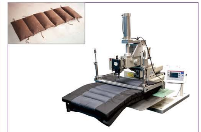
UN301542-2 Electronic pattern sewing machine with lifting head for sea cushions UN301542-2 Lifting height 150 mm, cushion diameter 840 mm
